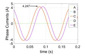
Figure 12. NATPOC condition fault-tolerant control currents.
