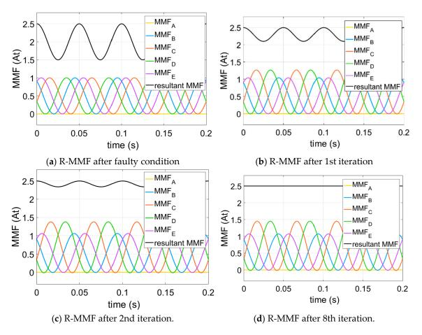
Figure 3. Single-phase open-circuit (SPOC) condition resultant MMFs.
