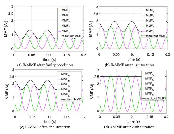
Figure 9. Adjacent three-phase open-circuit (ATPOC) condition resultant MMFs.
