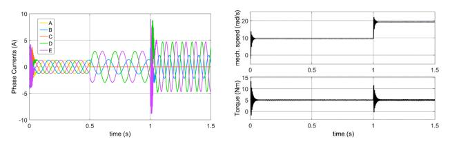
Figure 16. MATLAB/Simulink simulation results of the NADPOC fault-tolerant control currents.
