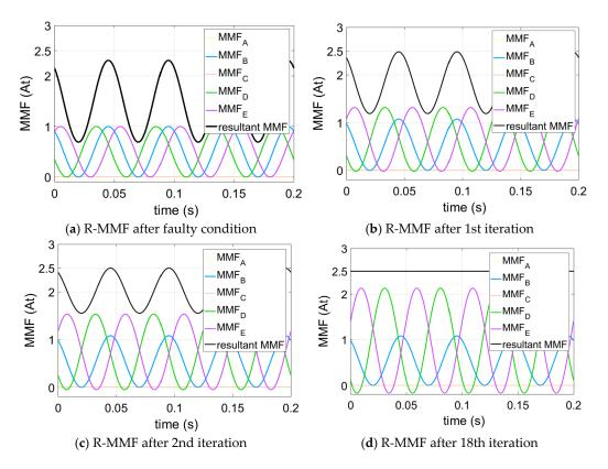
Figure 7. Non-adjacent double-phase open-circuit (NADPOC) condition resultant MMFs.
