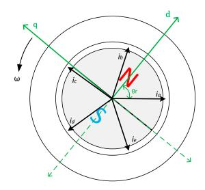
**Figure 1.** Illustration of the direct and quadrature (d-q) axes for the two-pole five-phase permanent magnet (PM) machine.
