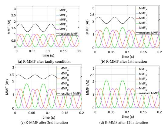
Figure 5. Adjacent double-phase open-circuit (ADPOC) condition resultant MMFs.
