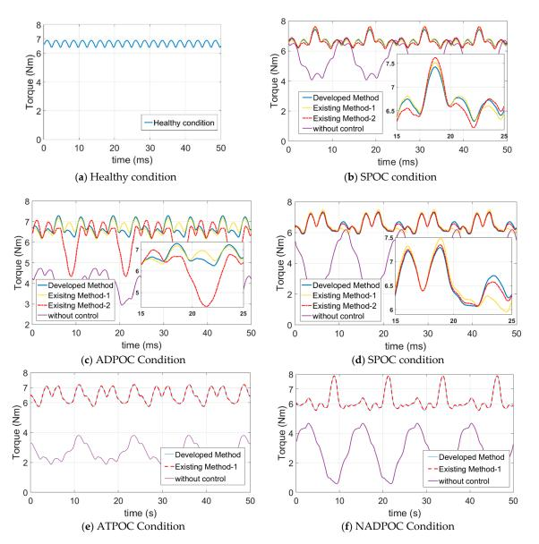
Figure 21. Model five-phase PM machine FEA torque results.
