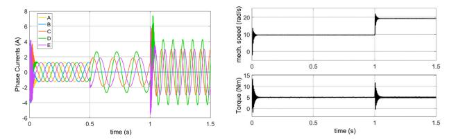
Figure 15. MATLAB/Simulink simulation results of the ADPOC fault-tolerant control currents.
