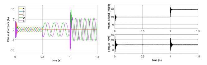
Figure 17. MATLAB/Simulink simulation results of the ATPOC fault-tolerant control currents.
