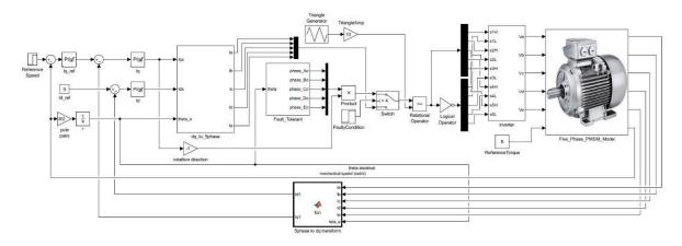
Figure 13. MATLAB/Simulink block diagram of the open-circuit fault-tolerant control.
