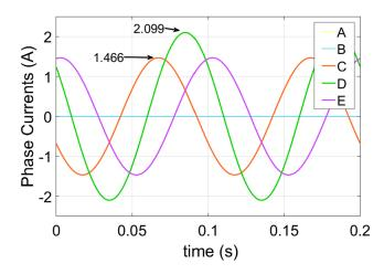
Figure 6. ADPOC condition fault-tolerant control currents.
