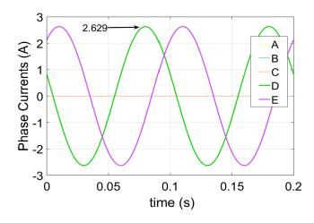
Figure 10. ATPOC condition fault-tolerant control currents.
