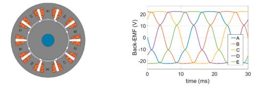
Figure 19. Modelled Five-phase PM machine and its back-EMF waveform.
