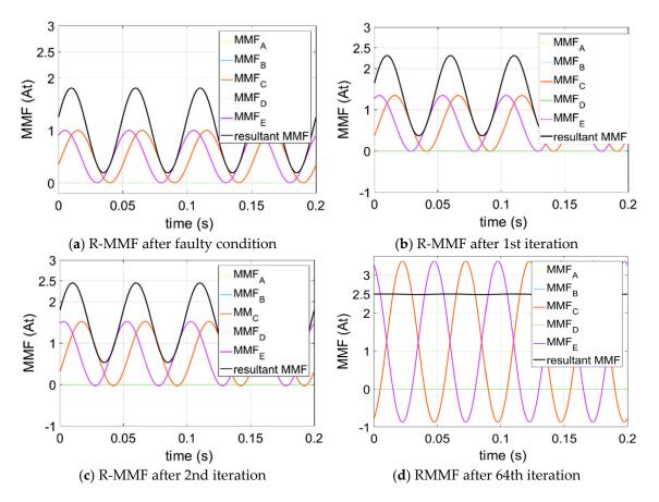
Figure 11. Non-adjacent three-phase open-circuit (NATPOC) condition resultant MMFs.
