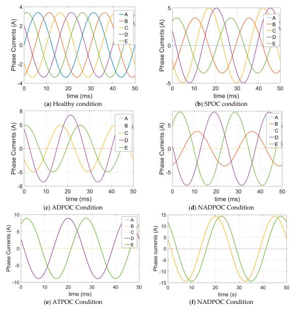
Figure 20. Model five-phase PM machine FEA current waveforms.
