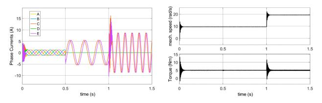
Figure 18. MATLAB/Simulink simulation results of the NATPOC fault-tolerant control currents.
