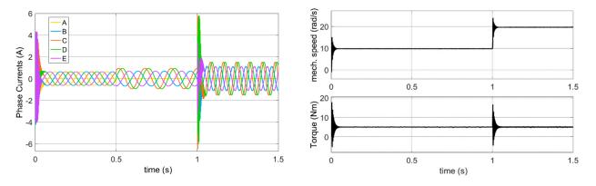
Figure 14. MATLAB/Simulink simulation results of the SPOC fault-tolerant control currents.
