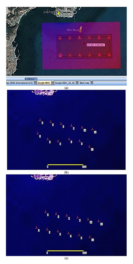
**Figure 8.** Optimal turbine layout for 12 WTGs (Wind Turbine Generators): (a) initial, (b) design of experiment (DOE) best solution (c) optimal solution.
