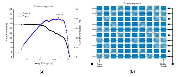
**Figure 3.** The output result for the  $10 \times 10$  PV array. (a) PV array without rearrangement. (b) The aging modules were covered with a plastic cap for clarification.
