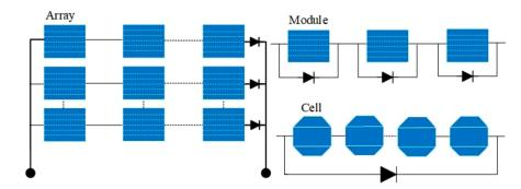
Figure 1. Componential structure of the photovoltaic (PV) array.
