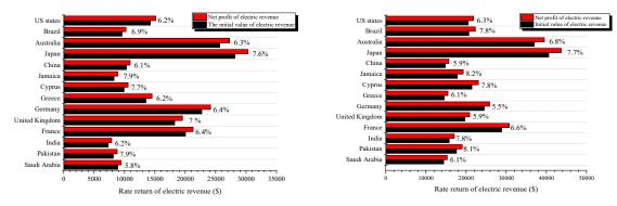
**Figure 14.** The increase in rate returns of electric revenue associated with the 18-kW and 43-kW  $10 \times 10$  PV arrays, taking into account the greatest economic advantage per year.
