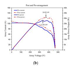
**Figure 13.** The outputs associated with the two types of  $10 \times 10$  PV arrays, namely, 18-kW (**a**) and 43-kW (**b**) before and after the implementation of reconfiguration.
