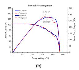
**Figure 10.** The outputs associated with the two types of  $10 \times 10$  PV arrays, namely, 18-kW (**a**) and 43-kW (**b**) before and after the implementation of reconfiguration.
