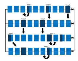
**Figure 6.** An example of the offline reconfiguration to swap PV modules through human labor in location.
