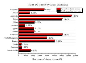
**Figure 11.** The increase in rate returns of electric revenue associated with the two types of  $10 \times 10$  PV arrays, taking into account the greatest annual economic advantage.
