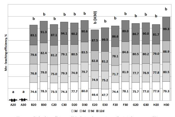
Figure 13. Bioleaching efficiency of Mn during the experiment (Statistical groups a and b).
