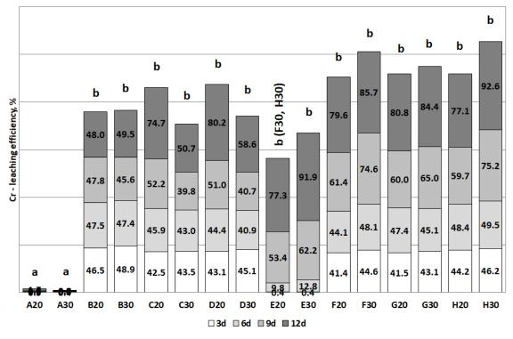
Figure 9. Bioleaching efficiency of Cr during the experiment (Statistical groups a and b).
