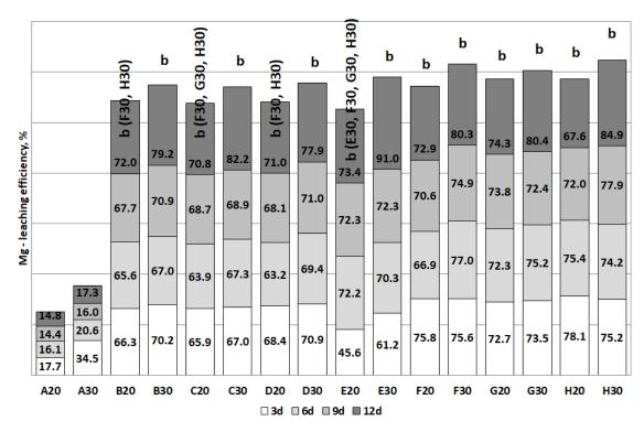
Figure 12. Bioleaching efficiency of Mg during the experiment (Statistical groups a and b).
