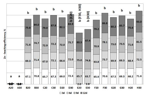
Figure 16. Bioleaching efficiency of Zn during the experiment (Statistical groups a and b).
