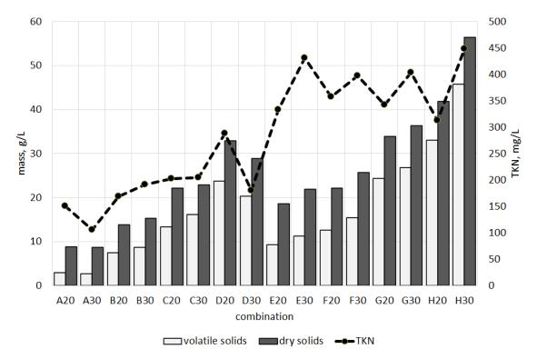
Figure 17. Mass balance during bioleaching for the tested combinations.
