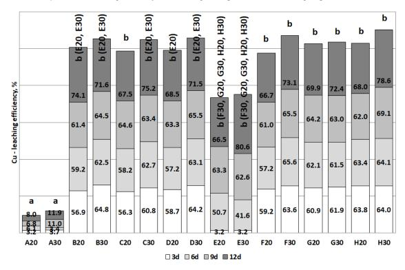
Figure 10. Bioleaching efficiency of Cu during the experiment (Statistical groups a and b).
