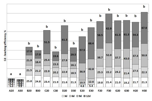
Figure 8. Bioleaching efficiency of Cd during the experiment (Statistical groups a and b).
