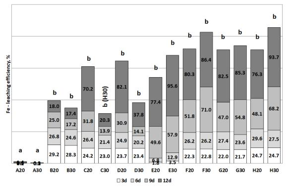
Figure 11. Bioleaching efficiency of Fe during the experiment (Statistical groups a and b).
