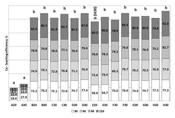
Figure 7. Bioleaching efficiency of Ca during the experiment (Statistical groups a and b).
