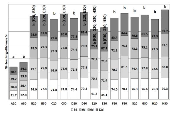
Figure 14. Bioleaching efficiency of Ni during the experiment (Statistical groups a and b).
