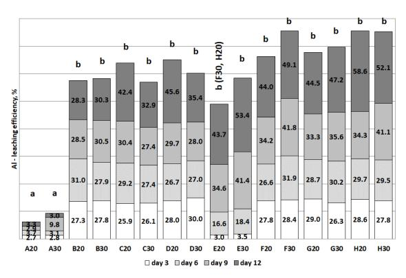
Figure 6. Bioleaching efficiency of Al during the experiment (Statistical groups a and b).
