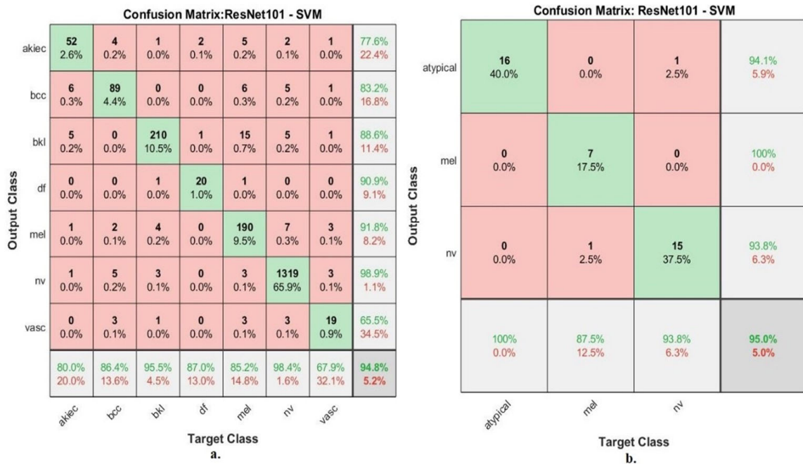
Figure 12. Confusion matrix for the classification of two skin lesion datasets by SVM with ResNet101 features through datasets of (a) HAM10000 and (b) PH2.
