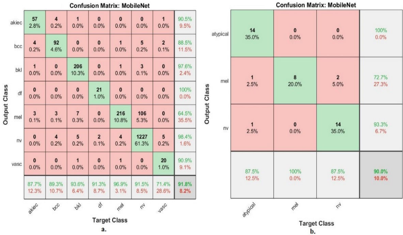
Figure 9. Confusion matrix for the classification of two skin lesion datasets by MobileNet through datasets of (a) HAM10000 and (b) PH2.
