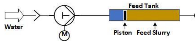
Figure 4. Pumping system of the LENA lab plant.
