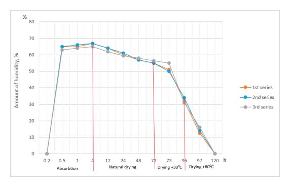
Figure 4. Drying process depending on the moisture content.
