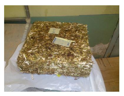
Figure 2. Slabs of hemp fibers with dimensions of  $300 \times 300$  mm.
