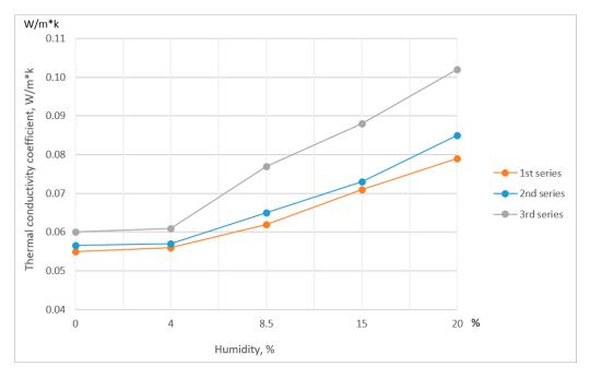
Figure 5. Thermal conductivity depending on the moisture content.
