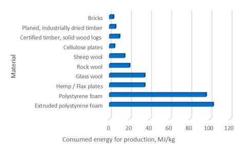
Figure 1. Consumed energy for thermal insulation and construction materials.
