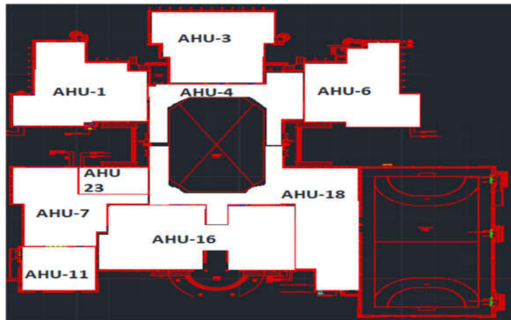
Figure A3. Air handling units in ground floor.
