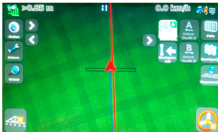
Figure 2. Image seen by the operator on the screen of the Trimble CFX 750 navigation panel—sample recording of the preset (red line) and actual (blue line) vehicle track.
