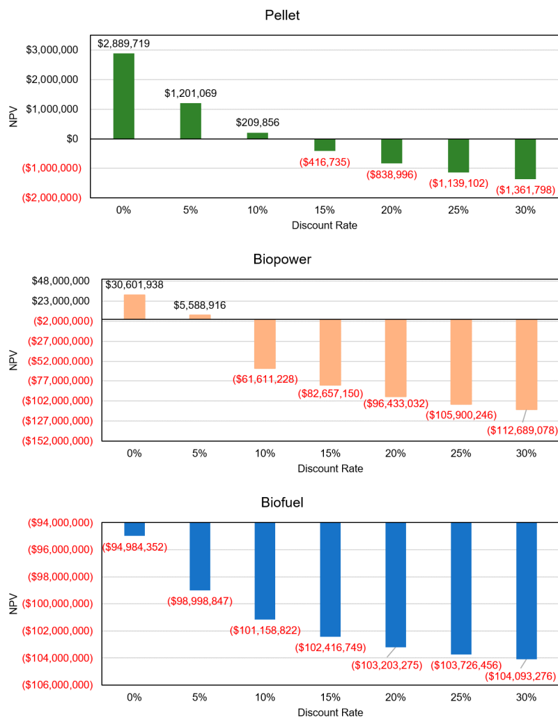
Figure 4. The impacts of discount rate on net present value for pellet, biopower, and biofuel production.
