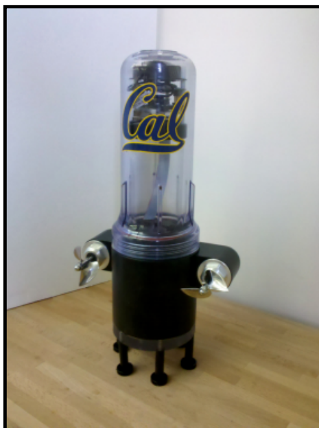
Figure 6. Generation 3 drifter floating sensor [18].
