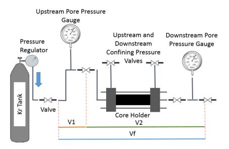
**Figure 3.** Pulse decay experimental setup for mass balance determination of gas storativity in rock. Setup is placed on a CT table for image acquisition after reaching pressure equilibrium for each pressure pulse.
