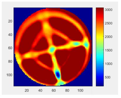
**Figure 7.** CT slice depicting the core and end cap boundary where the color scale reflects CT number in HU. The lighter (2000 HU range) areas reflect etching in the end caps that allows for a more distributed inflow of gas into the core. The changing CT numbers or density in these etched areas reflect the uneven contact surface between the rock and end cap. The low CT number (less dense) blue zone suggests that a void exists between end cap and core in that region.
