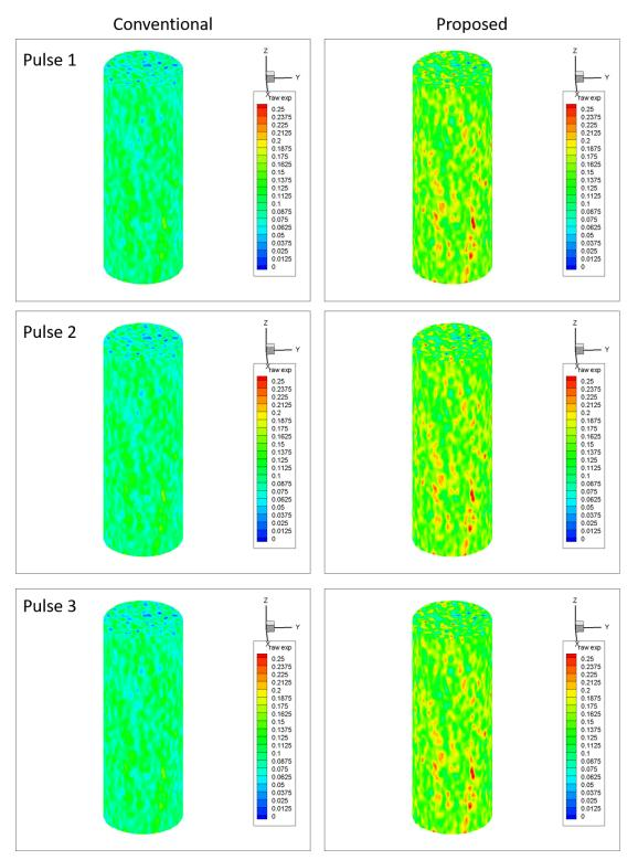
**Figure 8.** 3D CT images of Kr apparent porosity for the three pressure pulses conducted on the Wolfcamp sample. Local areas with relatively greater storage are consistent in both methods; however, the magnitude by which Kr stores in these areas differ.
