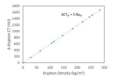
Figure 2. Pure Kr density versus  $\Delta$ CT at 20 °C scanned at 140 kV and 120 mA.
