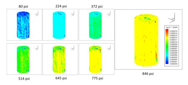
**Figure 6.** 3D CT images showing increasing Kr storage in the rock with pore pressure in the Eagle Ford sample. The color scale represents the mass of Kr in each voxel in Kg multiplied by the total number of voxels per slice, 10,545. Warmer colors indicate more gas in place.
