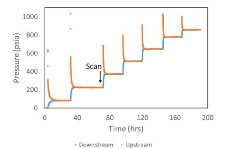
**Figure 4.** Pressure history of all Kr pressure pulses for the Eagle Ford sample. The black arrow illustrates that CT acquisitions are taken at the end of each pulse. This specific example shows a CT scan acquired at the end of Pulse 2. Slight unsteadiness in equilibrium pressure is observed in the last few pulses due to room temperature fluctuations that have greater influence at higher pressures.
