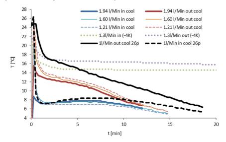
**Figure 8.** Temperature development during the discharging of the storage, in: Water temperature before the storage, out: Water temperature after the storage.
