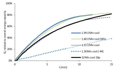
Figure 12. Released heat quantity during the discharging (in % of overall energy capacity of the systems).
