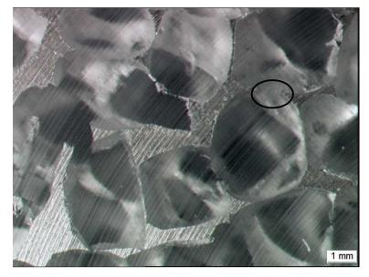
**Figure 15.** Cross-section of typical pore structure of aluminium foams used in the tests (for better visibility the picture was taken before removing the polymer placeholder, it is still in the structure). Connection window example marked with black circle.
