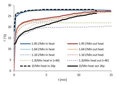
**Figure 7.** Temperature development during the charging of the storage, in: Water temperature before the storage, out: Water temperature after the storage.
