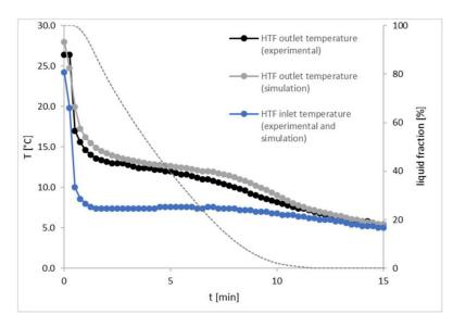
**Figure 13.** Comparison of the experimental and simulated outlet temperatures for the 4p-system, flow velocity 1.6 L/min.
