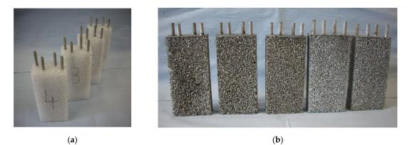
**Figure 3.** Polymer preforms (**a**) and open porous aluminum foams (**b**) with embedded tubes, for the 4p-system.
