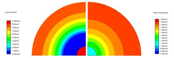
**Figure 14.** Comparison of the liquid fraction and temperature distribution at the cross-section of the modelled area at the middle of the pipe length of z = 1.2 m at t = 200 s.
