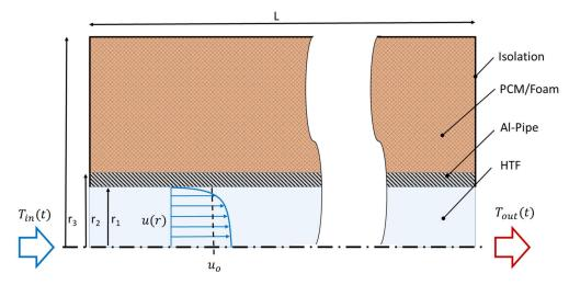
Figure 5. Geometrical simulation model.
