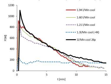
Figure 10. Power output from the storage during the discharging.
