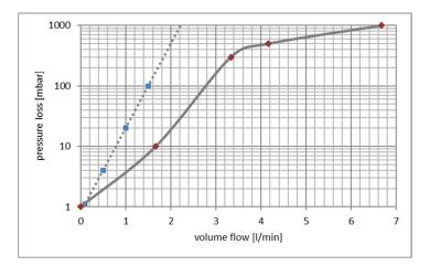
Figure 6. Pressure loss versus flow rate, dotted line: 26p, solid line: 4p.
