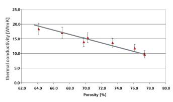
Figure 17. Dependence of thermal conductivity on Al foam porosity for the alloy AlSi9Cu3.
