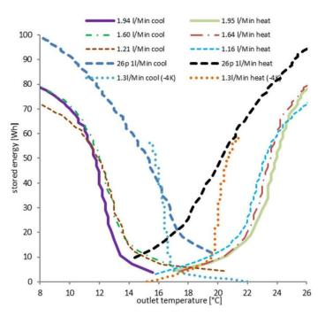
Figure 16. Delivered Heat Quantity depending on the temperature.
