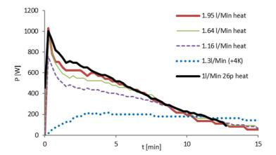
Figure 9. Power input into the storage during the charging.
