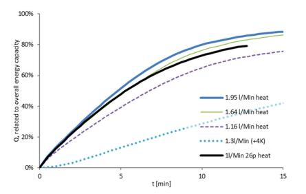
Figure 11. Stored heat quantity during the charging (in % of overall energy capacity of the systems).
