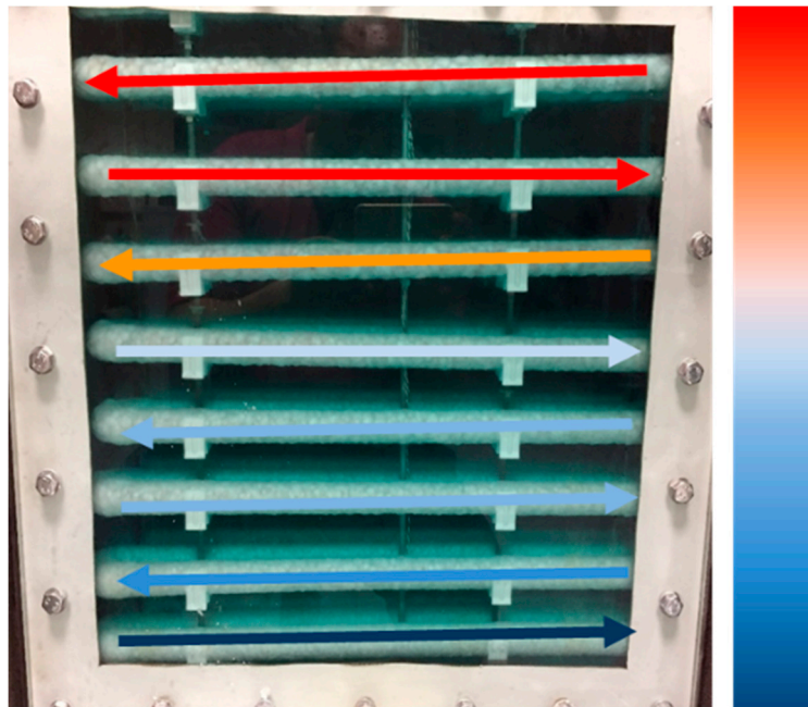
Figure 11. A photograph showing the solidification of the PCM on the tubes in the LHTESS during the discharging process.
