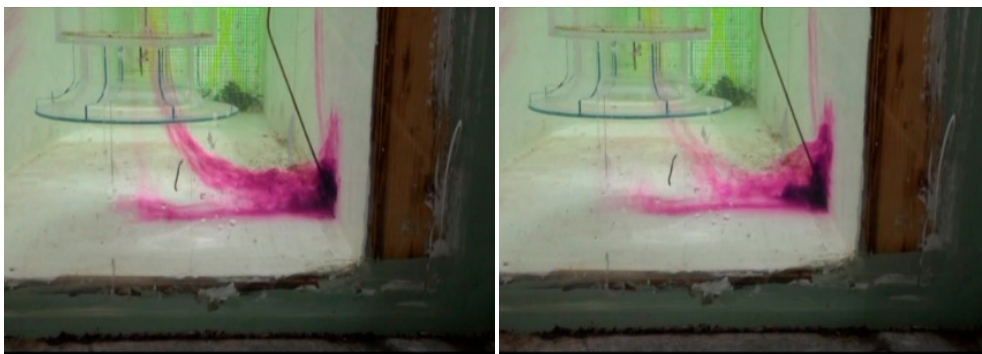
Figure 11. Intermittent side wall vortex. Type 1 to occasional type 3. Combined with the floor vortex increases the swirl along the pump column.
