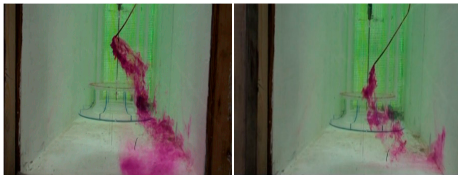
Figure 13. Flow instability and drifting behind the pump.
