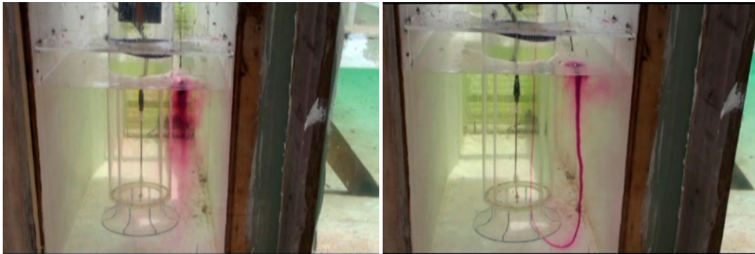
Figure 14. Image shows a free-surface vortex developing from a type 1 surface dimple (left) to a type 3 full dye core (right) vortex.
