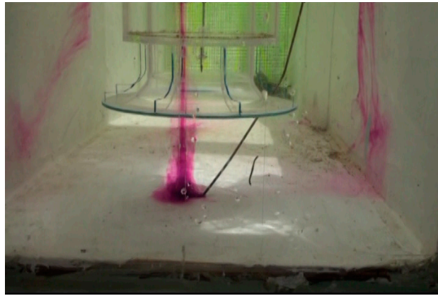
Figure 10. Strong type 2 floor vortex activity even with a maximum floor clearance of 0.5D (130 mm).
