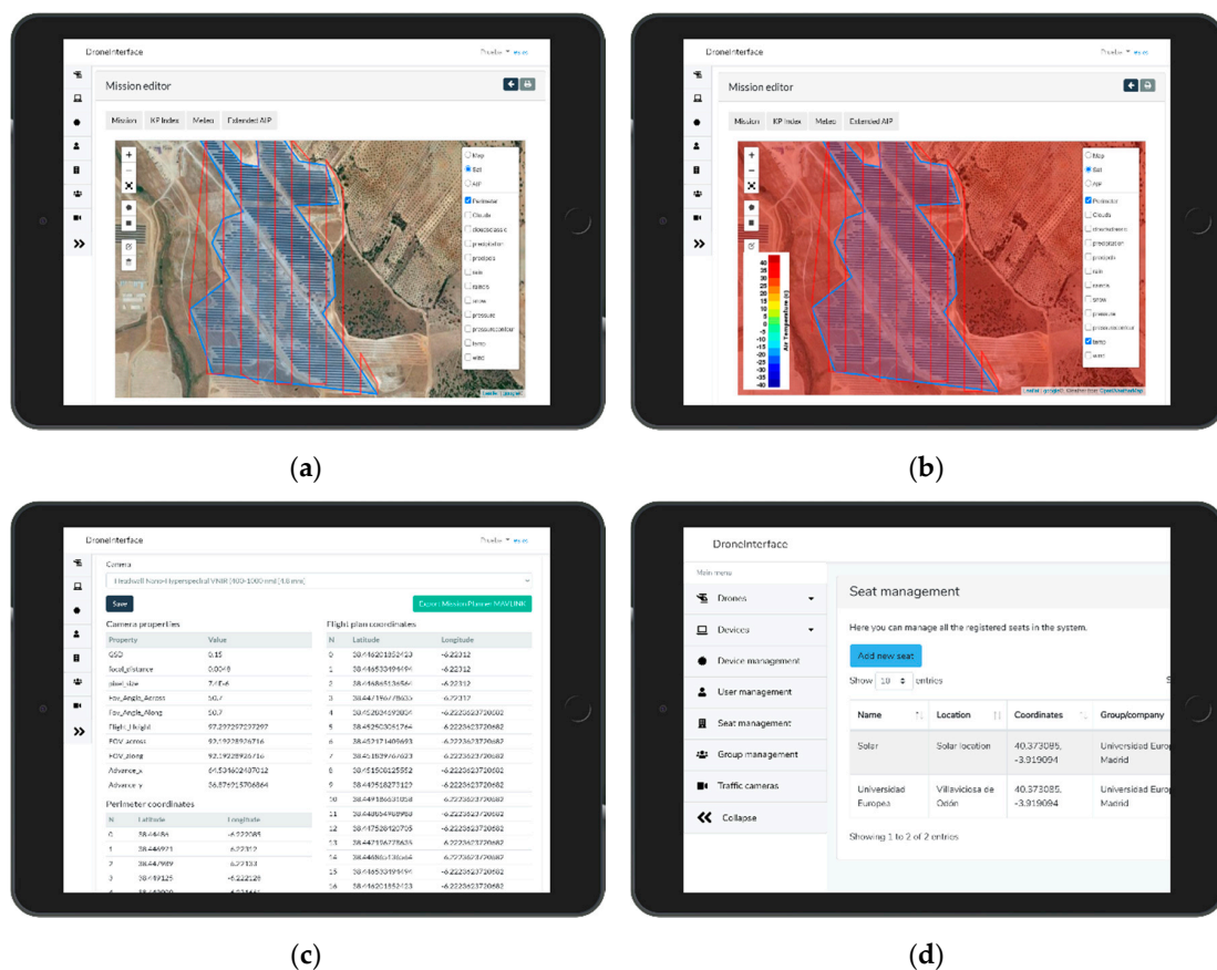
Figure 6. Screenshots of the application in different sections: (a) generation of inspection routes, (b) applying a meteorological observation layer relative to temperatures, (c) flight plans and data from the cameras, and (d) the management of locations for management.
