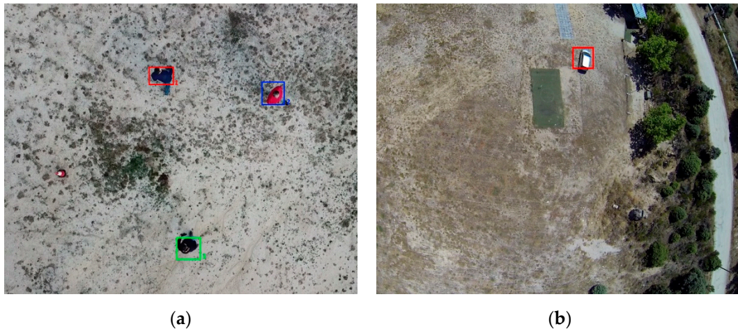
Figure 9. Object tracking algorithm on (a) pedestrians and (b) vehicles.
