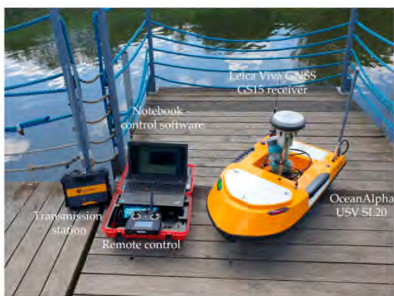
Figure 3. Unmanned Surface Vehicle (USV) with equipment for communication, data transmission and steering.
