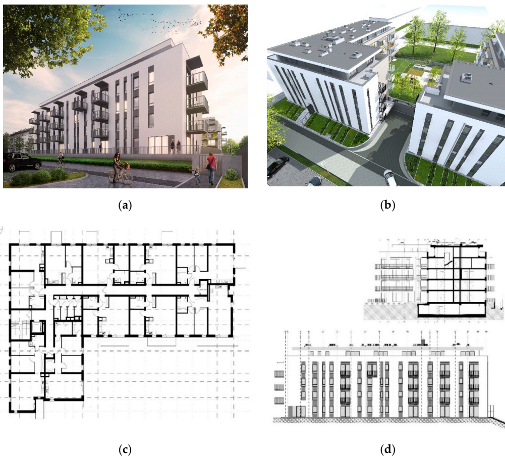
Figure 1. The building at Sadowskiego Street in Szczecin. (a) Visualization 01; (b) visualization 02; (c) floor plan; (d) cross section and east elevation.
