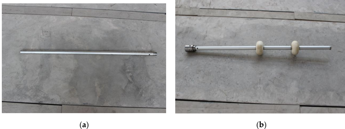
Figure 7. Typical pile structure: (a) P-1 equal-section pile; and (b) P-7 nodular pile.
