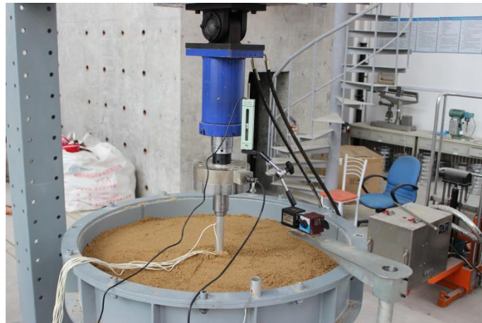
Figure 6. Dial indicator layout scheme.
