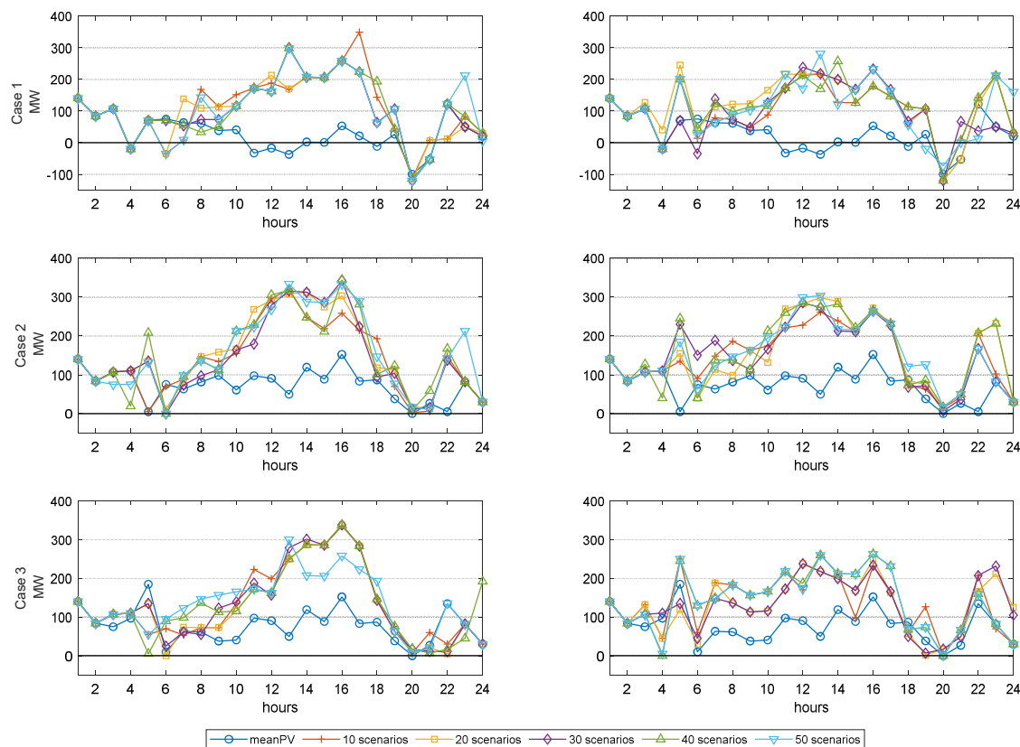
Figure 6. Difference between the feasible reserve schedule and minimum reserve from the results considering PV scenarios (left column) and PV load scenarios (right column) for cases 1, 2, and 3 (top to bottom).
