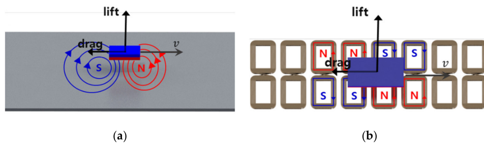
Figure 1. Induced current on two electrodynamic suspension (EDS) track types (Lift and drag forces act on the moving magnet on a (a) continuous sheet track and on a (b) discrete null-flux coil track).
