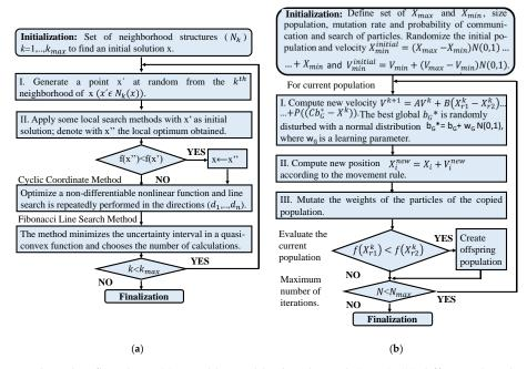
**Figure 1.** Algorithm flowchart: (**a**) variable neighborhood search (VNS); (**b**) differential evolutionary particle swarm optimization (DEEPSO). Code in detail available: http://www.gecad.isep.ipp.pt/WCCI2018-SG-COMPETITION/.
