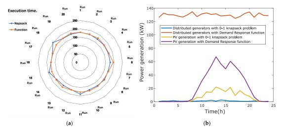
**Figure 12.** Results with the 0-1 KP and the DRF. (**a**) Execution time for 20 runs; (**b**) power exchanged by the electric vehicles (EVs) and the energy storage systems (ESSs).
