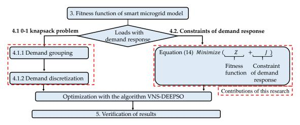
Figure 2. Conceptual formulation of a smart microgrid (SMG) with DR constraints.
