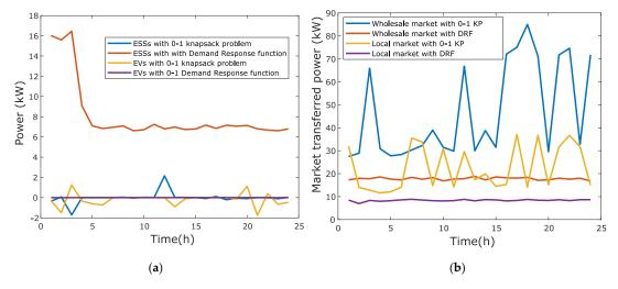
**Figure 13.** Power exchanged with 0-1 KP and DRF. (**a**) EVs and ESSs scheduling for day-ahead; (**b**) electricity markets scheduling for day-ahead.
