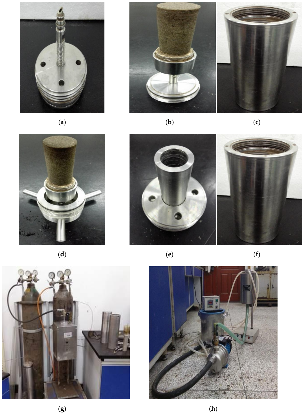
Figure 3. Physical diagram of mud cake forming device and flushing device. mud cake forming device: (a) is device cover, (b) is device lower cover, (c) is device outer, (g) is high-temperature and high-pressure filter; flushing device: (d) is device cover, (e) is device lower cover, (f) is device outer, (h) is physical drawing of flushing device.
