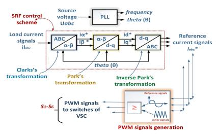
Figure 4. Synchronous Reference Frame (SRF) control scheme.
