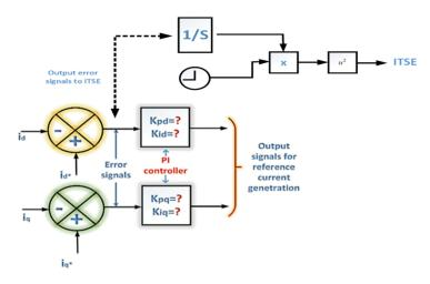
**Figure 5.** Proportional Integral (PI) controller loop with Integrated Time Square Error (ITSE) objective function block.
