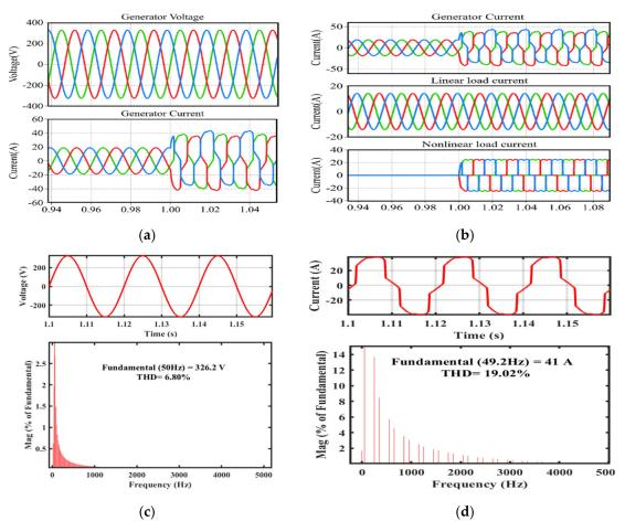
Figure 8. Overall results without control at point of common coupling (PCC): (a) generator voltage and current signals without control, (b) overall system current signals without control, (c) harmonics spectrum of generator voltage without control, (d) harmonics spectrum of generator current without control.
