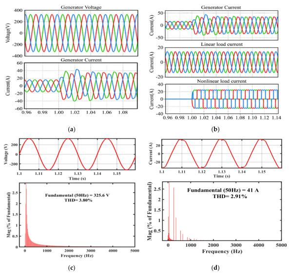
**Figure 10.** Overall results without control at PCC; (a) generator voltage and current signals with control; (b) overall system current signals with control; (c) harmonics spectrum of generator voltage with control; (d) harmonics spectrum of generator current with control.
