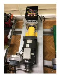
Figure 1. Tested generator with modified excitation system and driving DC machine.
