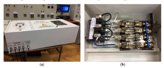
Figure 2. The outside (a) and inside (b) view on the short-circuit module.
