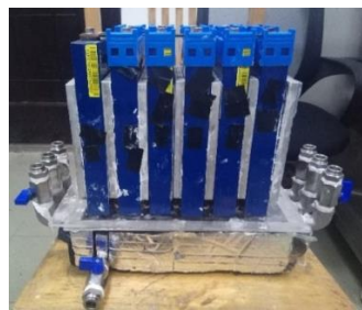
(a) Experimental model in CCCS (b) Installation drawing of aluminum plate, copper rods and heat sinks
