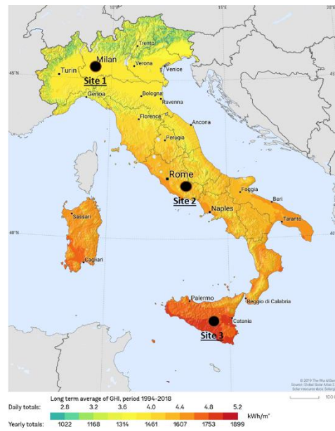
Figure 3. Global Irradiation map. Reproduced from [17], Global Solar Atlas: 2019.
