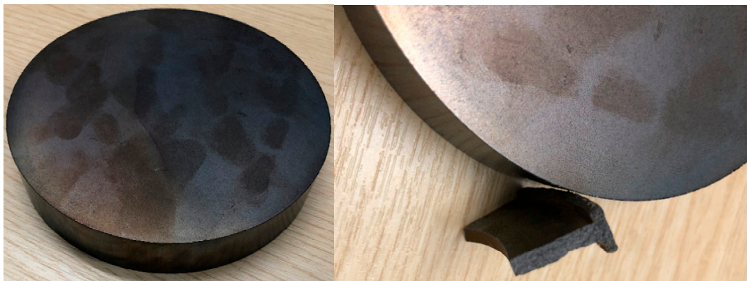
Figure 1. Commercially available Somaloy 700 HR 5P (by Höganäs) block by compression of SMC iron powder at 800 MPa (Outer dia.: 55 mm; height: 10 mm; \mu_{max} = 600 , B at 10,000 A/m is 1.57 T).
