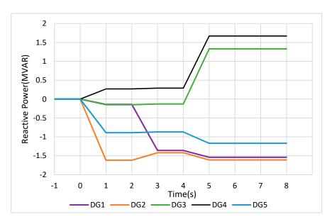
**Figure 12.** Generators reactive power response for scenario 3.
