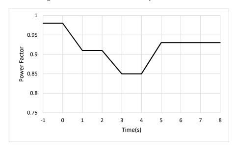
Figure 10. Power factor at the receiving/load end of the transmission line.
