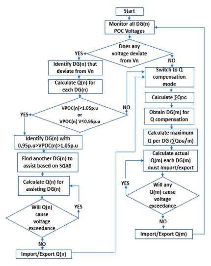
Figure 1. Proposed control algorithm flow chart.
