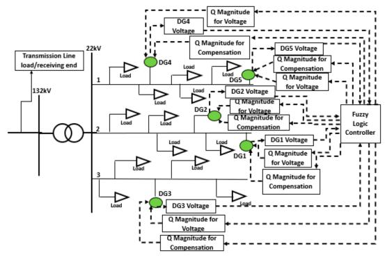
Figure 3. Distribution network with five generators and the controller interface.
