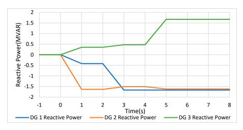
**Figure 8.** Distributed generator reactive power response for scenario 2.
