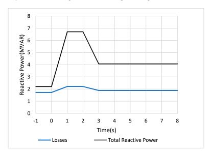
Figure 5. Transmission line total reactive power and losses for scenario 1.
