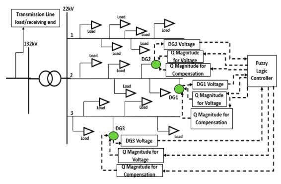
Figure 2. Distribution network with three generators and the controller interface.
