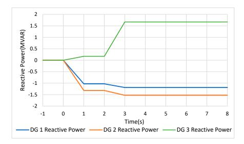
Figure 4. Distributed generators reactive power response for scenario 1.
