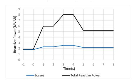
Figure 9. Transmission line total reactive power and losses.
