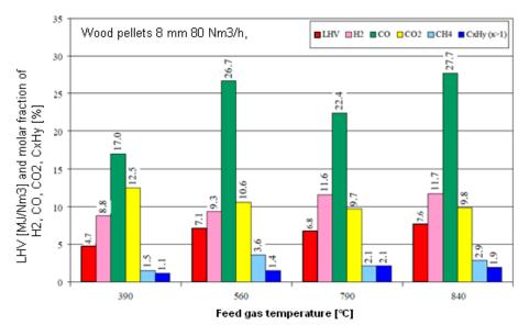
**Figure 13.** Influence of temperature of the feed gas on the average values of LHV and composition of dry fuel gas. Average values are taken from Phase II for batch type gasification 20 kg of 8 mm wood pellets.
