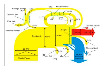
Figure 18. Sankey Diagrams—HiTAG/HiTSG Power Generation System.
