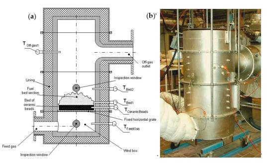
**Figure 6.** Side view of an updraft gasifier ( $T_{\text{Feed Gas}}$ —temperature of preheated feed gas,  $T_{\text{Bed1}}$ ;  $T_{\text{Bed2}}$ —reacting fixed-bed, fuel gas  $T_{\text{Off-gas1}}$  and ceramic beads  $T_{\text{Ceramic Beads}}$ ) (**a**), and batch type slag reactor HiTAG/HiTSG (**b**).
