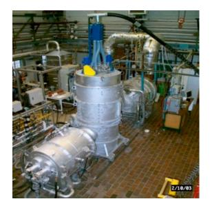
Figure 8. Experimental stand for continuous downdraft gasification.
