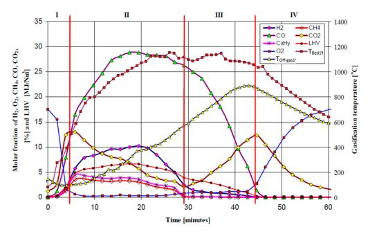
**Figure 9.** Changes of the fuel gas composition (H<sub>2</sub>, CO, CO<sub>2</sub>, CH<sub>4</sub>,  $C_xH_y$ , O<sub>2</sub>), LHV, gasifier bed temperature (T<sub>b1</sub>) and the exiting fuel gas temperature (T<sub>og1</sub>), versus gasification process time. Feed gas conditions: 50 Nm<sup>3</sup>/h of air preheated up to 350 °C (gasification 20 kg of 12 mm wood pellets).
