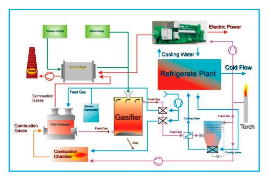
**Figure 17.** A proposal of a semi-industrial high-temperature biomass gasification installation for power generation design by KTH/GUT research group. The key component of the system is the FeG Preheater which produces a high-temperature feed gas.
