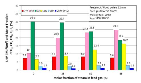
**Figure 14.** Influence of molar fraction of steam on the average values of composition and lower heating value of the fuel gas—gasification of 20 kg of 12 mm wood pellets (computed results).
