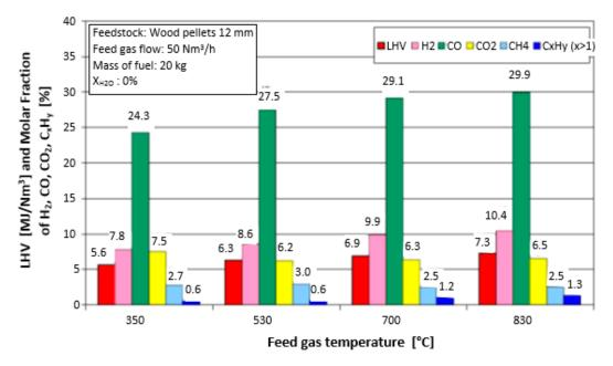
**Figure 10.** Influence of the feed gas temperature on the average values of LHV and composition of dry fuel gas (gasification 20 kg of 12 mm wood pellets—computed results).
