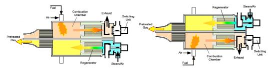
**Figure 2.** Concept of a high-temperature air/steam ceramic regenerator with a high-frequency alternating flow (with about 10–30 s for each mode) developed by Mochida and Hasegawa [5].
