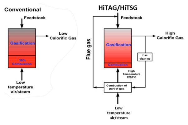
**Figure 4.** Comparison between conventional and HiTAG/HiTSG gasification. In the conventional system, the process involves lower temperatures (approx. 600–700 °C) and produces a low-calorific gas polluted with tars, ash, or even dioxin and furans. On the other hand, in the HiTAG/HiTSG system, ceramic regenerator allows obtaining high temperatures of the feed gas (flue gas) which produces high calorific and cleaner gas.
