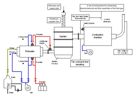
Figure 7. HiTAG/HiTSG test facility with a continuous gasifier.
