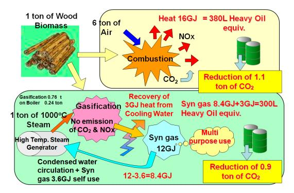
**Figure 16.** Example of effective utilization of biomass energy (Combustion and Gasification). Comparison of two methods: direct combustion (**top**) and gasification (**bottom**) shows a significant reduction of harmful pollutants.
