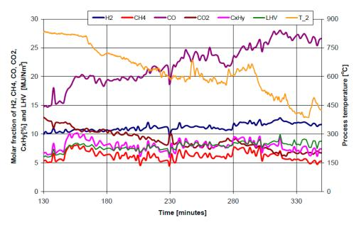
**Figure 11.** Composition, lower heating value and temperature of produced fuel gas in the gasification period of experiments.
