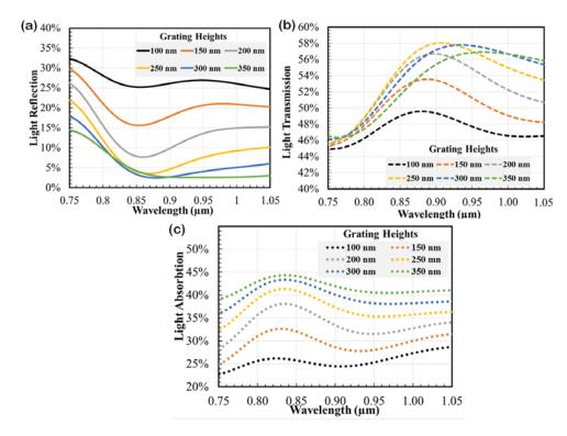
**Figure 5.** Observation of light reflection (a), transmission (b), and absorption (c) spectra for a triangular-shaped nano-grating structure with the grating pitch of 830 nm.
