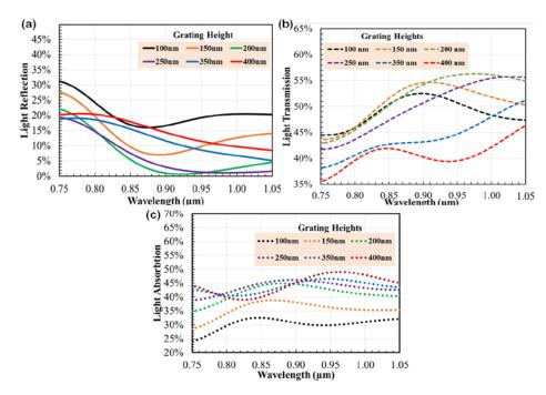
**Figure 6.** Observation of light reflection (a), transmission (b), and absorption (c) spectra for a trapezoidal-shaped nano-grating structure. The aspect ratio for the trapezoidal structure was 0.5.
