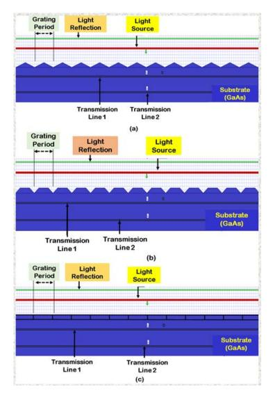
**Figure 4.** Simulation plane diagrams of (a) triangular-shaped nano-gratings with the aspect ratio of zero, (b) trapezoidal-shaped nano-gratings with the aspect ratio of 0.5 and (c) rectangular-shaped nano-gratings with the aspect ratio of one, on top of the semiconductor (GaAs) substrates.
