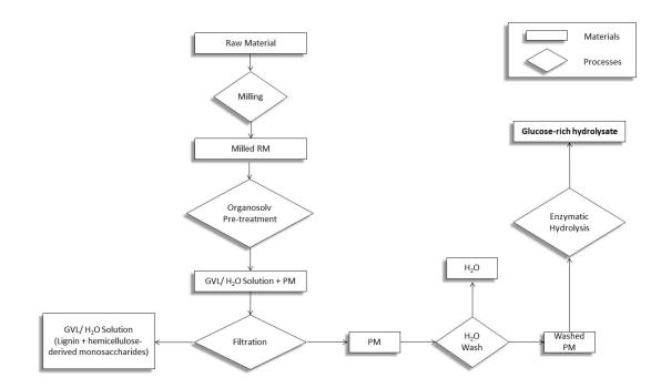
Figure 1. Flowchart of the overall process for the production of fermentable glucose.
