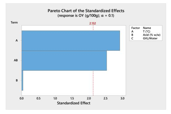
**Figure 2.** Pareto chart for the OY response, the dashed line indicates the significance limit of the factors on the response.
