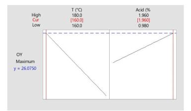
**Figure 4.** The optimization plot shows the conditions needed to maximize the OY. The vertical red lines on the graph represent the current factors' (temperature and acid concentration) settings.
