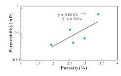
Figure 4. The correlation between porosity and permeability of P<sub>1</sub>t sandstone.
