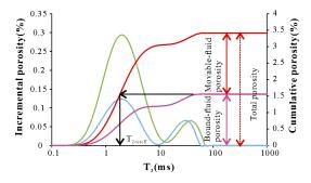
Figure 6. The cumulative and incremental T<sub>2</sub> spectrum of sample 5.
