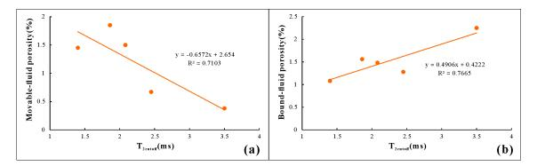
**Figure 12.** The correlations between movable-fluid porosity, bound-fluid porosity and  $T_{2cutoff}$ . (a) the correlation between  $T_{2cutoff}$  with movable-fluid porosity; (b) the correlation between  $T_{2cutoff}$  with bound-fluid porosity.
