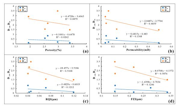
**Figure 10.** The correlations between petrophysical parameters with multifractal parameters. (a) the correlations between  $D_{-10}$ ,  $D_{10}$  with porosity; (b) the correlations between  $D_{-10}$ ,  $D_{10}$  with permeability; (c) the correlations between  $D_{-10}$ ,  $D_{10}$  with RQI; (d) the correlations between  $D_{-10}$ ,  $D_{10}$  with FZI.
