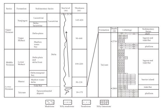
**Figure 2.** Map showing the stratigraphic column of Permian successions in the SNCB (modified from [38]) and more details of Taiyuan Formation (well wc1), including burial depth, lithology, sedimentary facies.
