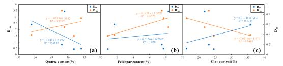
**Figure 13.** The correlations between mineral compositions and multifractal parameters. (a) the correlations between  $D_{-10}$ ,  $D_{10}$  with quartz content; (b) the correlations between  $D_{-10}$ ,  $D_{10}$  with feldspar content; (c) the correlations between  $D_{-10}$ ,  $D_{10}$  with clay content.
