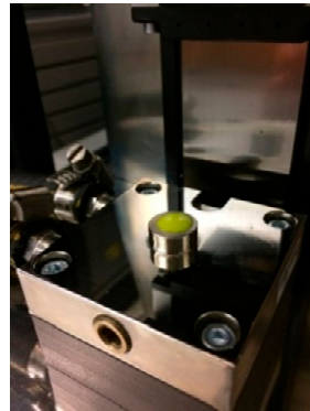
Figure 10. One of our custom-made phosphor samples on the measurement stage of a Mentor DynTIM (dynamic thermal interface material thermal conductivity measurement) equipment [45].
