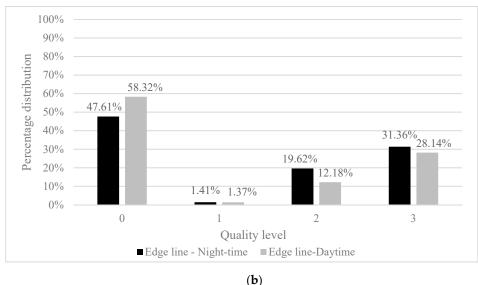
**Figure 2.** Comparison of the Mobileye readings (quality level) between night-time and daytime quality measurements for middle (**a**) and edge lines (**b**).
