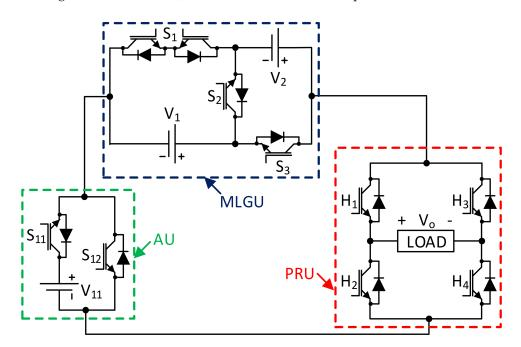
Figure 1. Proposed hybrid inverter topology.
