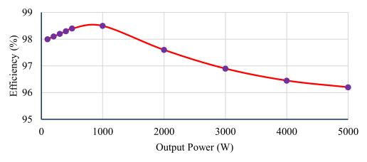
Figure 5. Efficiency plot of the proposed topology.
