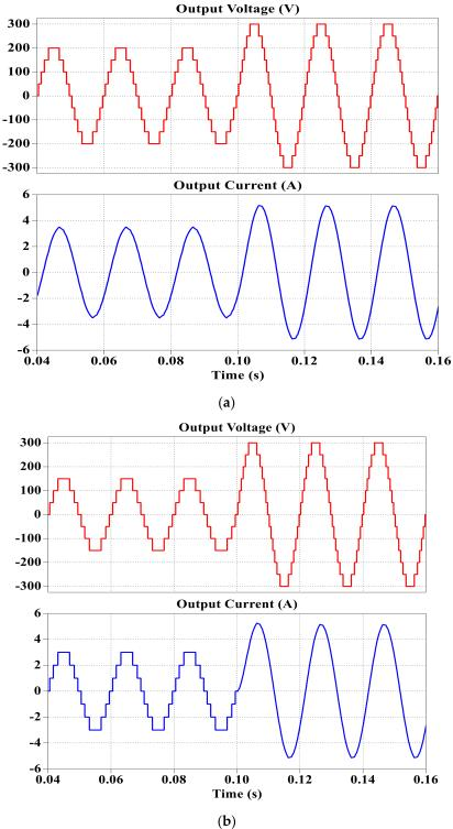
**Figure 8.** Terminal voltage and Load current for (**a**) change of MI with R-L load and (**b**) change of MI and load from R load to R-L load.
