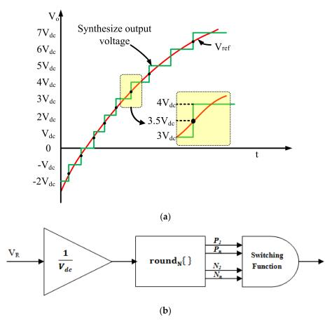
**Figure 4.** NLCPWM with (**a**) Synthesizing the Terminal Voltage from Reference (**b**) Switching Function of NLM method.
