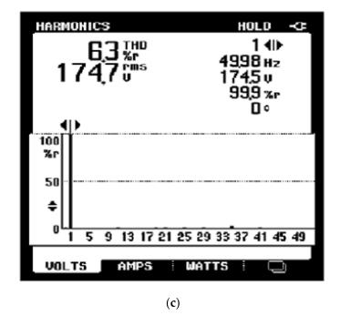
**Figure 10.** Terminal voltage and Load current for (**a**) R load and (**b**) R-L load, and (**c**) harmonic spectrum of output voltage.
