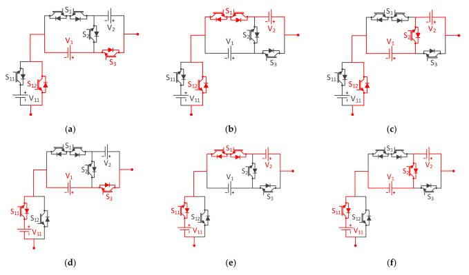
**Figure 2.** Different switching states of level generation unit (**a**)  $V_o = V_1$ , (**b**)  $V_o = V_2$ , (**c**)  $V_o = V_1 + V_2$ , (**d**)  $V_o = V_{11} + V_1$ , (**e**)  $V_o = V_{11} + V_2$ , and (**f**)  $V_o = V_{11} + V_1 + V_2$ .
