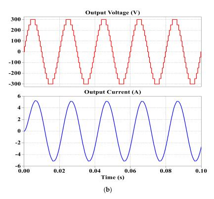
**Figure 7.** Simulation results (**a**) Terminal voltage and Load current for R load. (**b**) Terminal voltage and Load current for R-L load.
