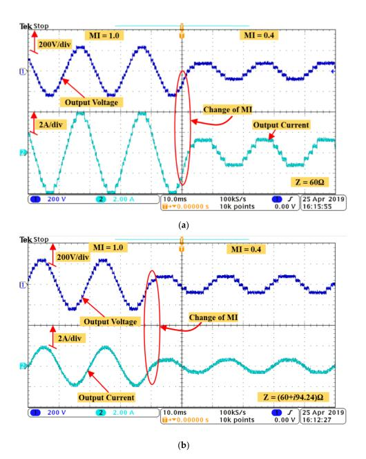
Figure 11. Terminal voltage and Load current with a change of MI with (a) R load and (b) R-L load.
