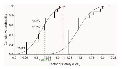
**Figure 13.** Graph of the lower and upper bounds of cumulative probability of factor of safety approximated by normal distribution functions.
