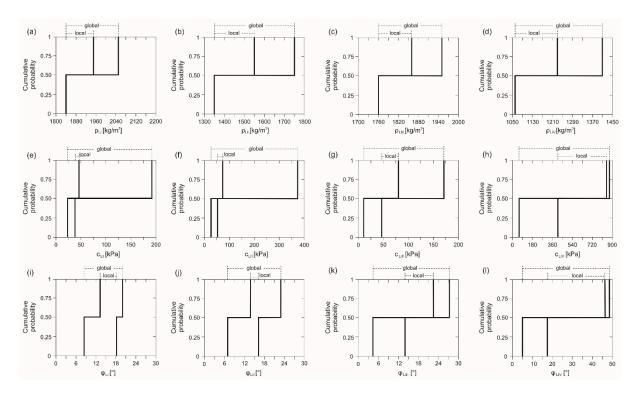
**Figure 9.** Input data–bulk density, cohesion, and internal friction angle presented as random sets for lithological units: (**a**,**e**,**i**) LI; (**b**,**f**,**j**) LII; (**c**,**g**,**k**) LIII; (**d**,**h**,**l**) LIV.
