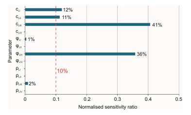
**Figure 10.** Sensitivity diagram of parameters adopted for the numerical stability analysis of the 18S landslide in the Bełchatów open-pit mine.
