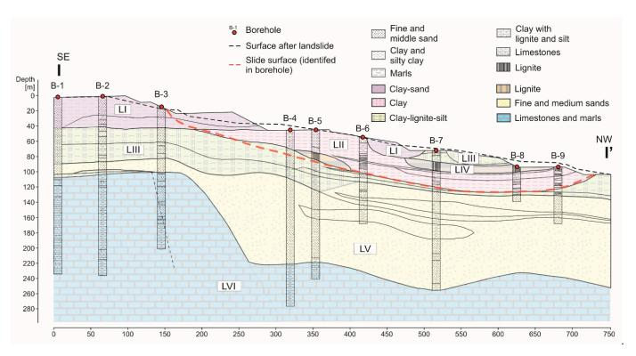
Based on the distinguished lithological units, a cross section was made along the longitudinal axis of the landslide, which was used for numerical calculations (Figure 8).
