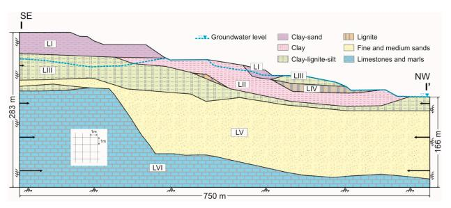
Figure 11. Calculation model of the 18S landslide in the Bełchatów open-pit mine.
