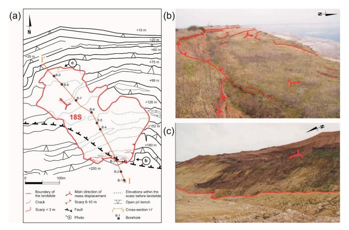
**Figure 3.** (a) Sketch of 18S landslide; (b) crown and main scarp of the landslide on the level +205 m a.s.l.; (c) colluvium fragment on the level +78 m (photo by R. Kaczmarczyk).
