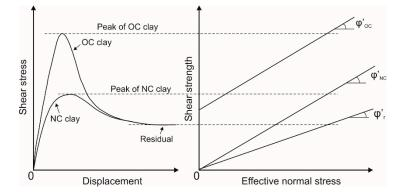
**Figure 1.** Stress-displacement curves (left-hand side) and failure lines of over-consolidated (OC) and normal consolidated (NC) clay (right-hand side), (based on [9]); description in the text.
