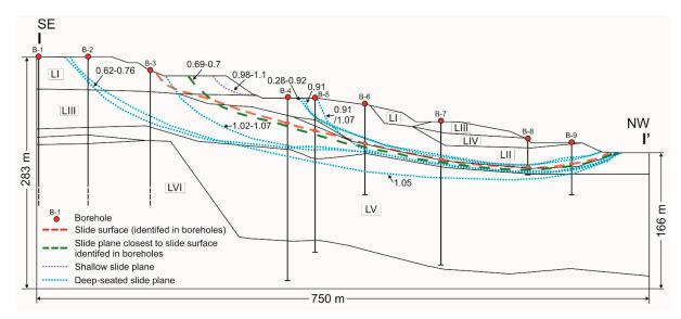
Figure 12. Location of the generalised slide planes with assigned factors of safety less than 1.1 and slide surface identified in boreholes.
