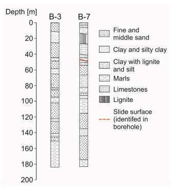
**Figure 4.** Characteristic geological profiles based on B-3 and B-7 boreholes in the region of the 18S landslide in the Belchatów mine.
