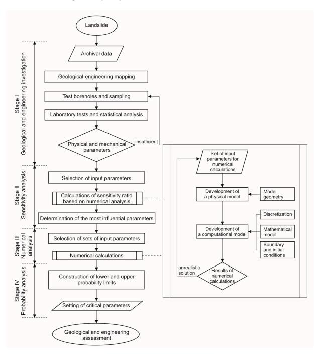
Figure 5. Scheme of the research methodology for the 18S landslide in the slope of the Bełchatów open-pit mine.
