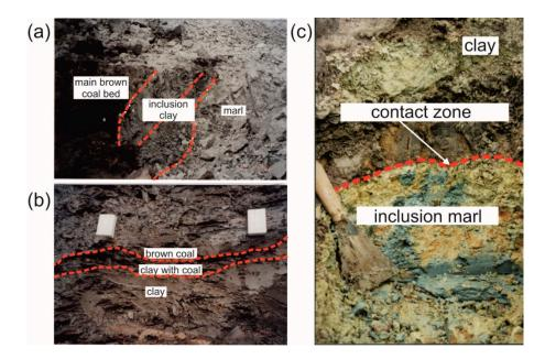
**Figure 6.** An example view of the complex structure and properties of the colluvium in the research area: (**a**) visible clay inclusions in the main lignite seam A; (**b**) contact zone between lignite and clay; (**c**) waterlogged contact zone between clay and marl (photo by R. Kaczmarczyk).
