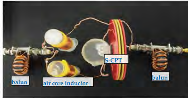
Figure 17. Experimental setup of the S-CPT system.
