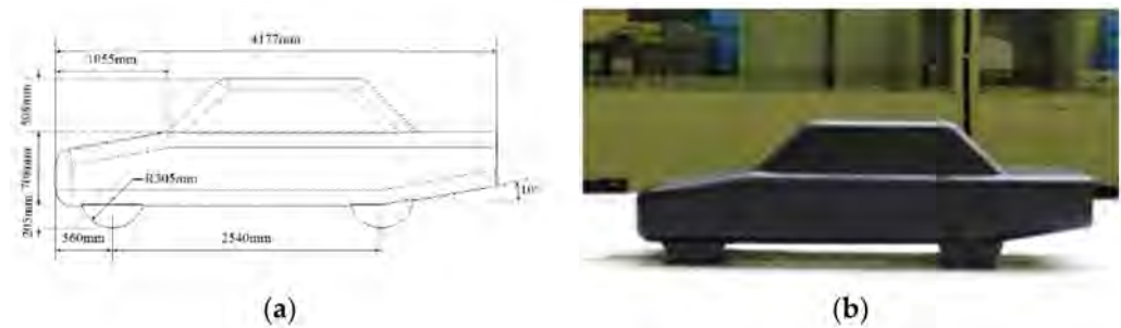
Figure 1. (a) Original size of MIRA notch back model; (b) 1/8 scale test mode in wind tunnel.
