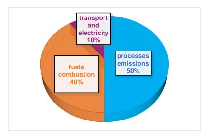
Figure 1. Operations in which CO<sub>2</sub> is generated in the OPC production process [49].
