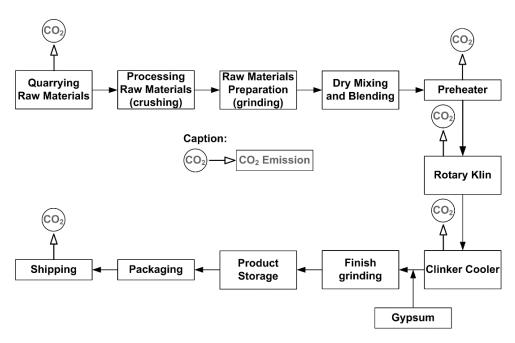
Figure 2. Detailed diagram showing the steps of OPC manufacturing and stages during which CO<sub>2</sub> is emitted [49].
