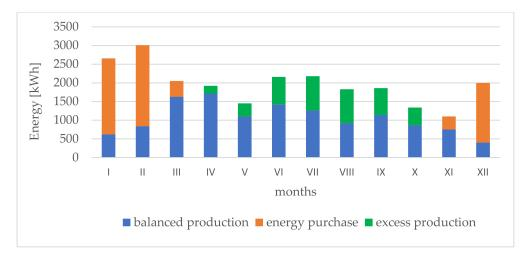
**Figure 3.** Summary of monthly electricity production in PV installation with an electric power of 18 kW with pump energy consumption heat with a power of 25 kW thermal power. Source: own study.
