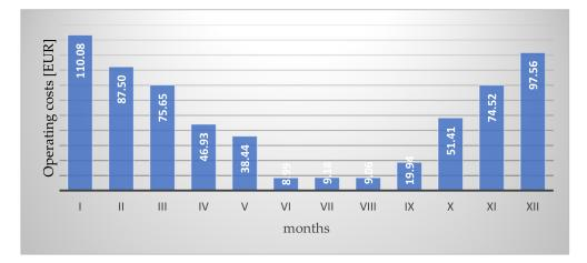
**Figure 2.** Summary of monthly costs for the electricity used to drive the heat pump compressor. Source: own study.
