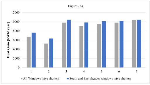
**Figure 11.** The total energy consumption (**a**) and heat addition (**b**) for the first case scenario: all windows have shutters and second case scenario: south and east windows have shutters with seven different windows shutter mechanism.
