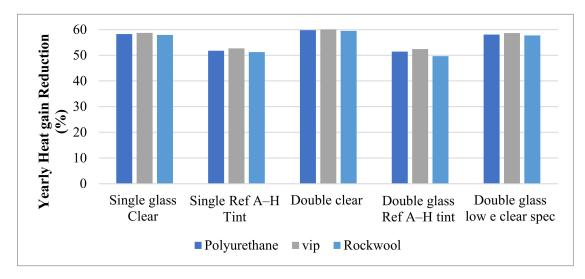
**Figure 6.** Yearly reduction in the total heat gain through different types of window glass applying three types of window shutters' insulations.
