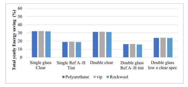
**Figure 7.** Yearly reduction in the total energy consumption of the building applying different types of window glass integrating three types of window shutters' insulations.
