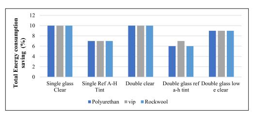
**Figure 10.** Total energy saving for different types of window glass with the three types of window shutters' insulations applying the glare with index 18.
