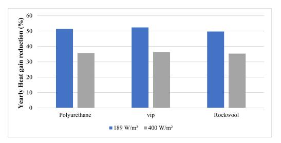
**Figure 8.** Yearly reduction in the heat gain of the building applying different types of window glass integrating three types of window shutters' insulations for different solar intensities.
