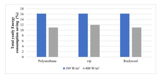
**Figure 9.** Yearly reduction in the total energy consumption of the building applying different types of window glass integrating three types of window shutters' insulations for different solar intensities.
