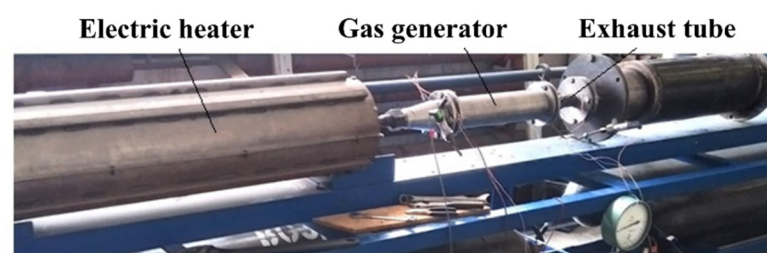
Figure 2. Direct-connect scheme of flow-through GG.
