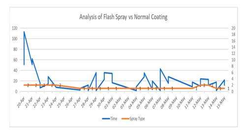
**Figure 14.** Analysis downtime due to tablet feed issues of Flash Spray (a 22-min spray) vs. Full Spray (a 72 min spray) showed no difference in downtime because of the two spray types over the 4 weeks of the analysis. Flash Spray type 2 used from 21 April to 27 April and 13 May to 16 May and Normal Spray Type 1 utilized from 28 April to 12 May.
