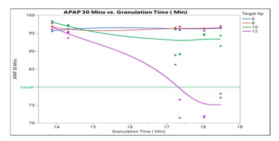
product will fail on dissolution testing. An increase to 12 KP ensured over 50% sampled failed batch testing for dissolution of the tablet.
