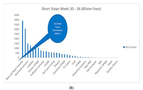
**Figure 20.** (a) Before the project started and actions were implemented, tab feed stops or downtime associated with tab feeds was the top downtime issue; (b) After the project implemented corrective actions, the tab fed issue was eliminated as a contributor to short stops or downtime.
