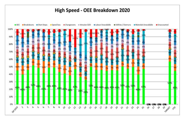
**Figure 3.** Packaging bar graphs of downtime issues/losses within the Packaging department with % OEE on the x-axis compared against Time (in weeks) on the y-axis. Breakdowns, Short Stops, Changeovers, Labor unavailable, Material Unavailable, Utilities/Overruns, Speed loss, Intrusive stops were all identified as sources of losses in downtime as demonstrated in the bar graph.
