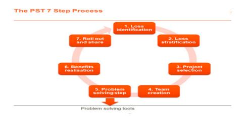
**Figure 1.** A seven-step in-company problem solving framework: based on and integrated with the Six Sigma D,M,A,I, C methodology and utilizing Lean and Six Sigma tools.
