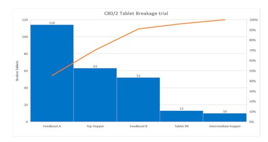
**Figure 13.** Pareto graph demonstrating the results of a trial to establish when tablets break within the Packaging process. It was demonstrated that 70% of breakages of tablet type C80/2 were in the Feed Bowl and Top hopper areas.
