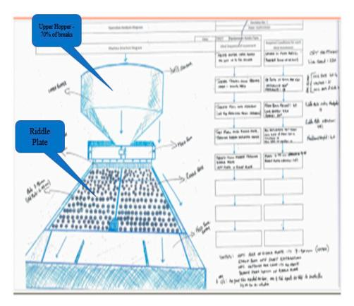
Figure 19. POA and pilot on a tailor-made product-specific riddle plate to understand how the plate would work. A new riddle plate was trialed on the C08/2 line whilst running 10C821 tablet type.
