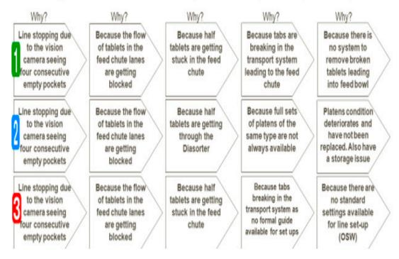
**Figure 17.** Five Whys analysis being conducted on the tablet feed issue led to root cause and corrective actions which addressed the reason for feed issues and tables getting broken or stuck.
