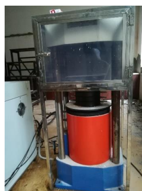
Figure 2. Electro-hydraulic servo compression testing machine.
