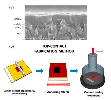
**Figure 1.** Top-contact fabrication method: (a) Cross-sectional scanning electron microscopy (SEM) image showing the MAPbI<sub>3</sub> layer with large grains and a flat interface with the electron-transporting layer (ETL); (b) Schematic of top-contact fabrication on a perovskite solar cell (PSC) and successive vacuum curing treatment.
