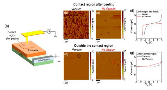
**Figure 4.** Conductive atomic force microscopy (CAFM) measurements: (a) Schematic of conductive atomic force microscopy (CAFM) measurements; Current maps (b), (c) and local intensity current-voltage (I-V) measurements (d) in the region of the contact after peeling for DBv-PSC and for DB-PSC. Current maps (e), (f) and local I-V measurements, in the areas indicated by black (DBv-PSC) and red (DB-PSC) circles, outside the contact region (g). The maps are taken at a fixed voltage of 3 V.
