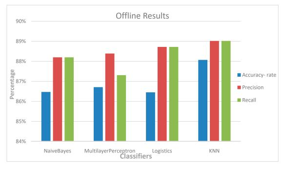
probabilistic model. In a real-time environment, the results showed that the KNN model performed better predictions regarding the status of the bin, as shown in Figure 8.
