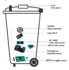
Figure 3. Smart bin used in SGCS.
