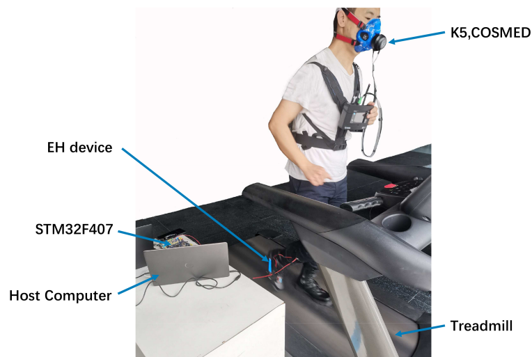
Figure 5. The subject walks on a treadmill at different speed of 4 km/h, 5 km/h, 6 km/h, 7 km/h, and 8 km/h, respectively. The K5 is used to monitor the rate of Oxygen consumption and Carbon dioxide production. An ADC of STM32F407 is used to record the voltage of resistor.
