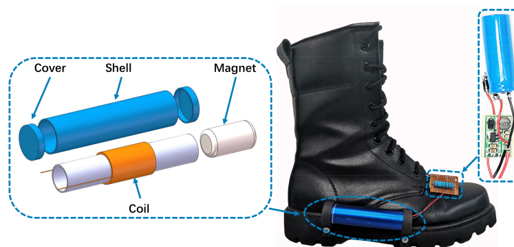
Figure 2. Energy harvesting device. The device is installed on the shoe. During the swing period of the gait, the magnet cuts the coil to generate an induced electromotive force, and the generated electrical energy is stored in the fast charging battery through the voltage stabilizing circuit.
