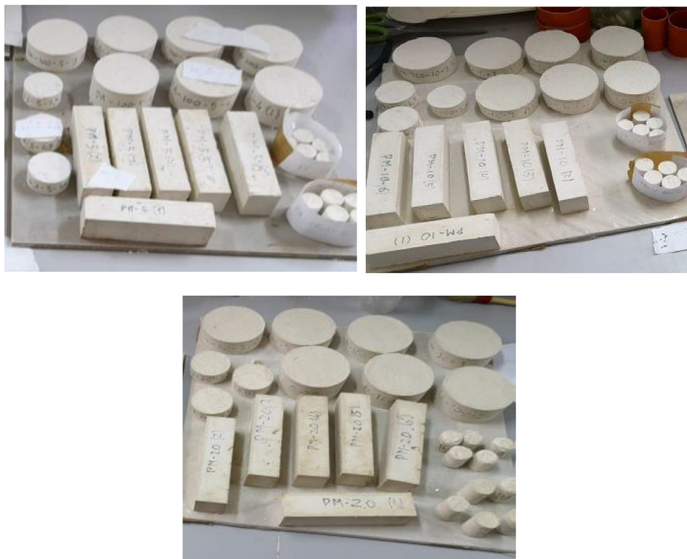
Figure 2. Specimens disarmed (5%, 10% and 20%, respectively).
