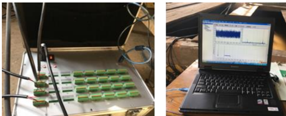
Figure 20. Test instruments of pressure fluctuation.
