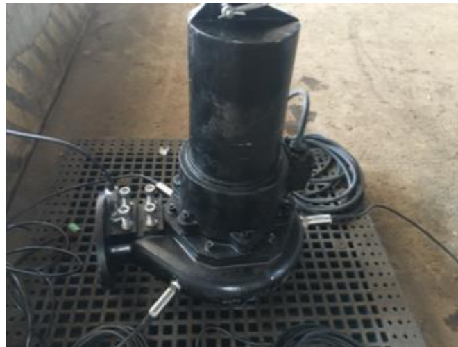
Figure 21. Test pump installed pressure sensors.
